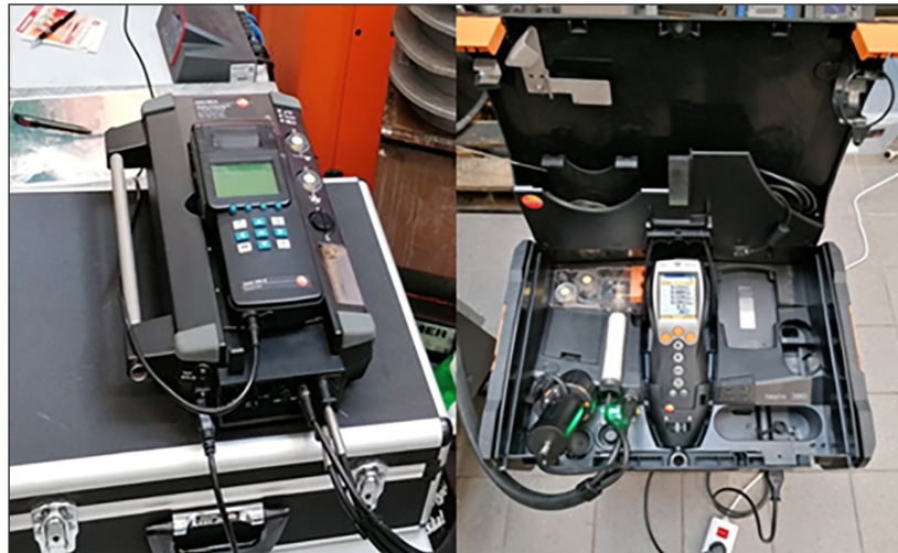
Fig. 2. Flue gas analyzers used in the tests: Testo 350S (left), Testo 330-2 LL (right)
